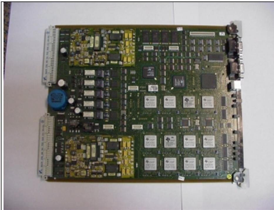
This board with 10 layers (board B of table II) includes many BGA and QFP with pin spacing of 50 mil and less. The combination of boundary scan test and flying probe test produces a minimal saving of 39% on the number of test steps.
