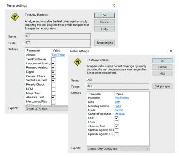
**TestWay Express** handles cross optimization along the test line, such as Boundary-Scan or AOI, that can be used to minimize the cost of In-Circuit Test or Flying Probe Test.
