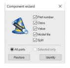
A component wizard is provided to simplify the component modeling, automatically identifying device classes, importing any available models and extracting valuable component information, such as value, tolerance, shape etc, directly from the BOM description.
