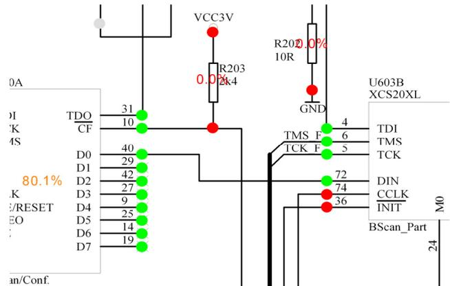
TestWay also allows users to reconstruct “virtual schematics” directly from a netlist, providing a navigation capability that includes advanced graphical symbols to identify board interconnections.
