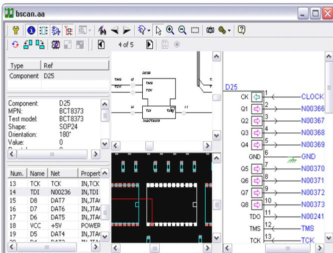
QuadView provides visualization of test coverage and customer attributes in both the schematic and layout views to clearly identify pin and device coverage, such as a green dot for covered and a red dot for uncovered pins.
