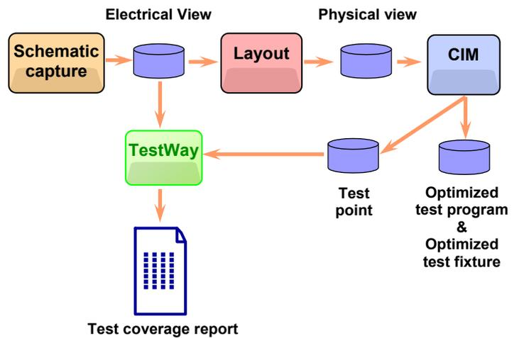
TestWay produces a testability report, written in a natural language that can be used by design and test engineers to validate that specific DfT criteria have been implemented.
